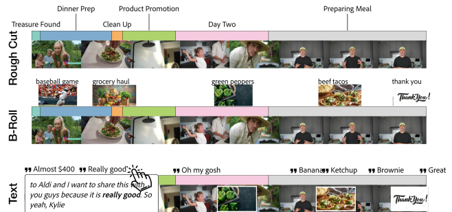
Figure 3: At each editing stage, VideoDiff provides glanceable timelines for users to easily compare different variations. Users can click on any section, B-roll image, or text effect to jump to that part of the video and preview the effects.
